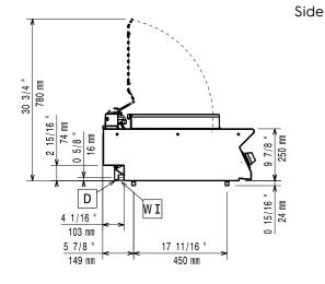
Drain Electrical inlet (power) ΕI
